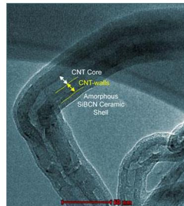
Figure 1 A Composite Structure of Ceramic Material and Carbon Nanotubes.
