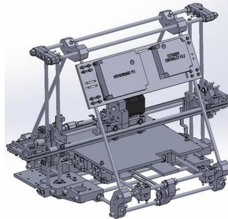
*Figure 3 A Reprap Mendel Prusa 3D Printer*
